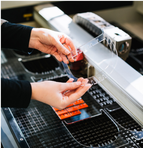
Design technology students have access to a wide variety of rapid prototyping equipment such as laser cutters.
