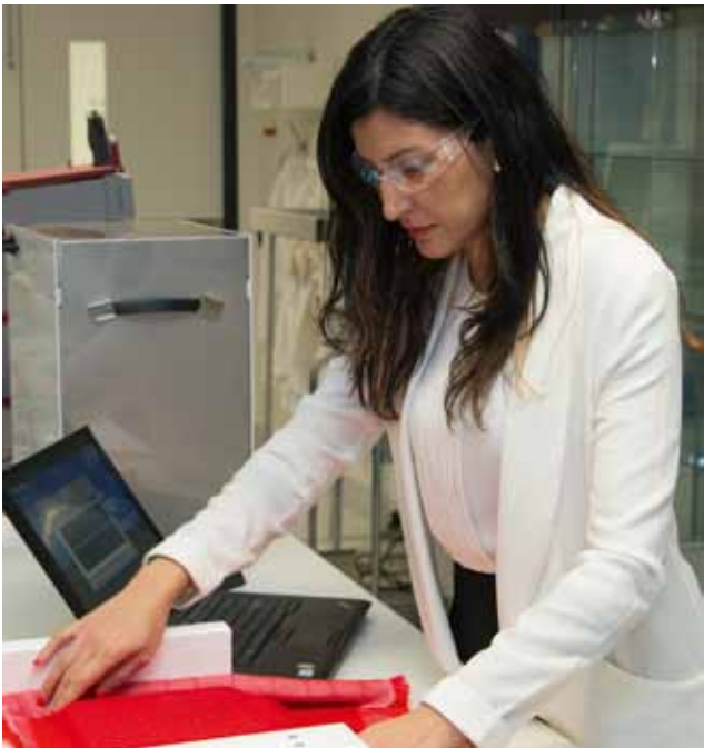
> Dr Maryam Naebe investigates the comfort properties of different fabrics using the Wool Comfort Meter.
