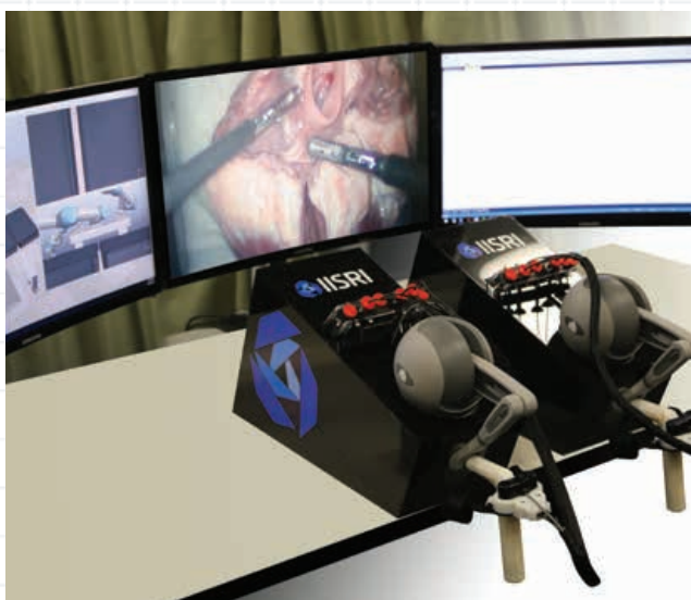
Top right: The key feature of haptic feedback will enable improved diagnosis and treatment. Above: Extra views of the surgical site will help surgeons see the instruments and laparoscope in 3D space.
