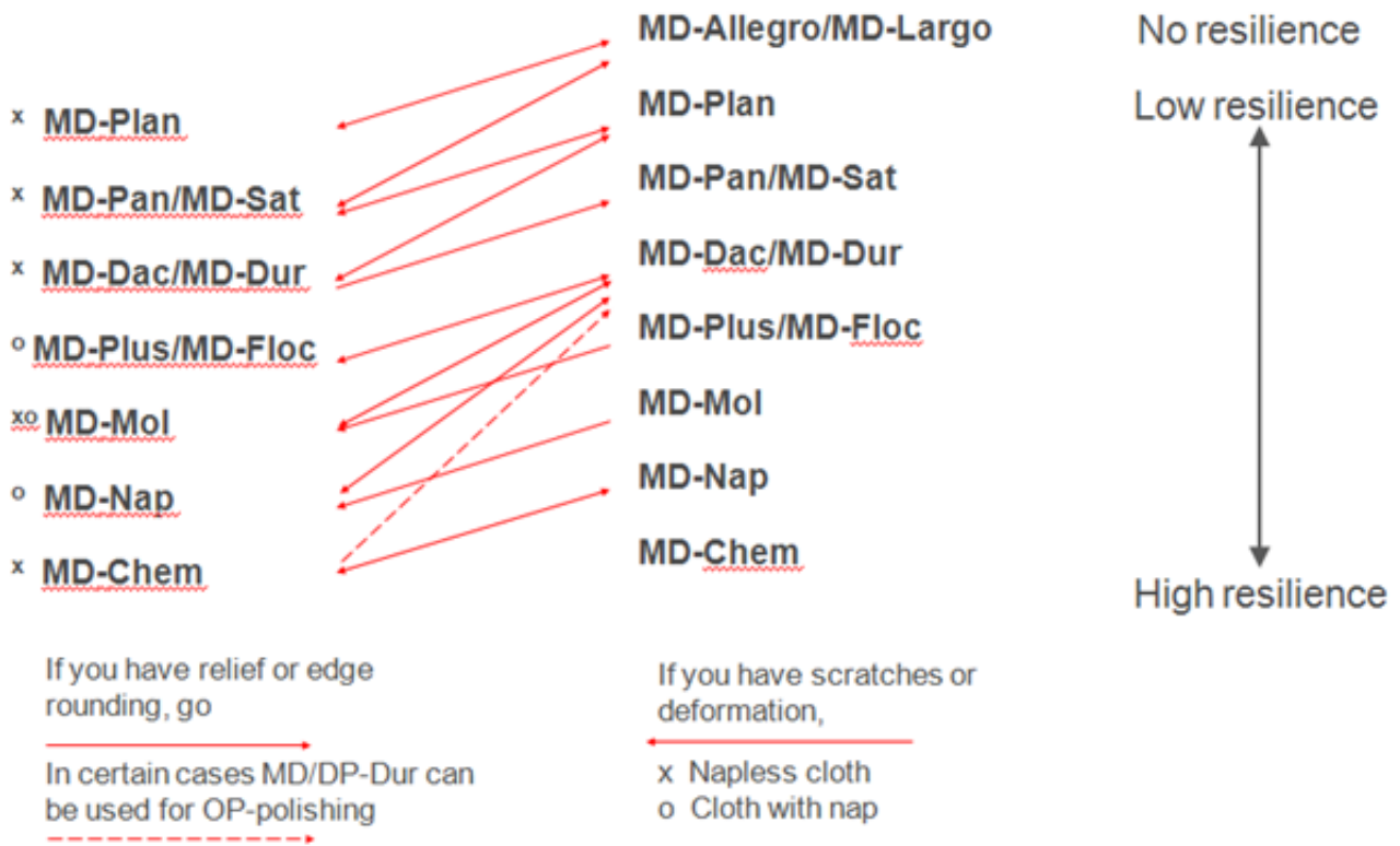
FIGURE 7: TROUBLESHOOTING GUIDE FOR MD-DISCS AND MD-CLOTHS WHEN METHOD DOESN'T PRODUCE HIGH QUALITY SURFACE OF THE SPECIMEN.
