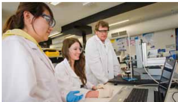
Researchers using the Scanning Electrochemical Microscope to probe the electrochemical response of new corrosion inhibitors for magnesium alloys.
