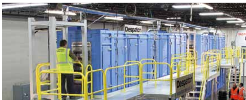
The carbon fibre processing line.
