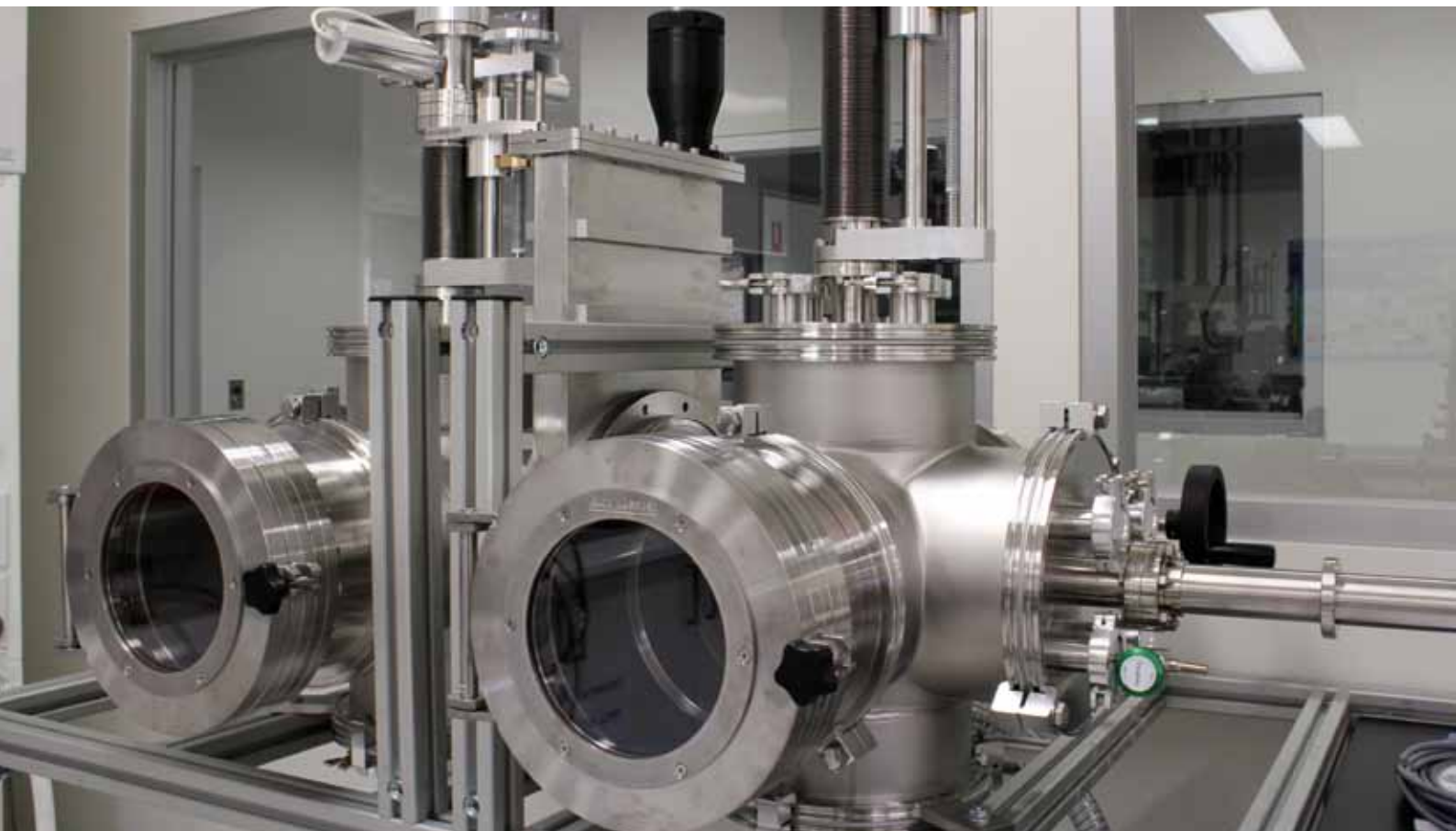
The custom designed advanced plasma facility combines physical vapour deposition with plasma enhanced chemical vapour deposition in a dual-chamber system.
