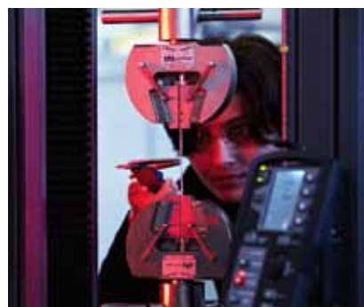
Tensile testing of a wrought magnesium alloy.
