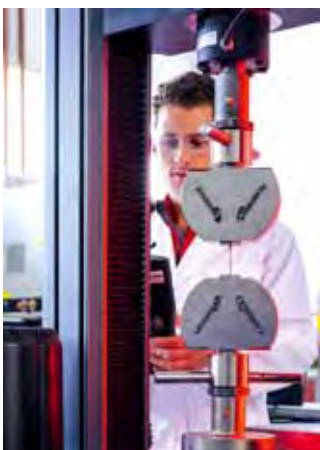
PhD student Andreas Kupke uses the Instron mechanical tester to perform tensile tests.
