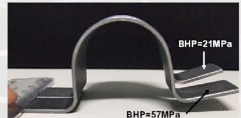
Comparison of springback in an advanced high strength steel for two process windows. Image: Tim De Souza
