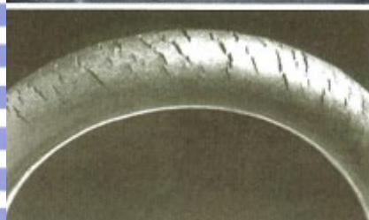
Ozone cracking in natural rubber tubing.
