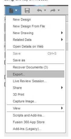
This open the dialogue page for exporting part file to another location such as a thumb drive. Using the drop-down arrow under 'Type:' select IGES File. Selecting the '...' next to original file location will open 'File browser' to choose location for part to be saved to, eg Thumb-drive. Then simply hit 'Save' and IGES will be created in designated file.
