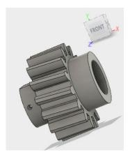
With Fusion 360 part needs to be assigned to home position on coordinates, this is start from 0 point of axis's. The Part still requires to be orientated in the ZY plane. This can either be from beginning of modelling or on completion through the Move Function.
