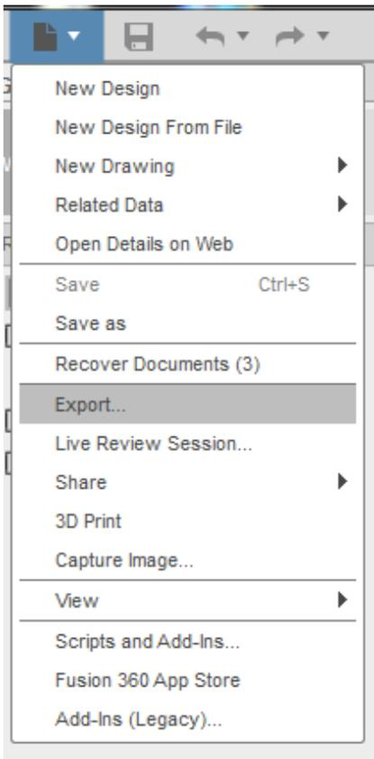
This opens the dialogue page for exporting part file to another location such as a thumb drive. Using the drop-down arrow under '**Type:**' select IGES File. Selecting the '...' next to original file location will open '**File browser**' to choose location for part to be saved to, eg Thumb-drive. Then simply hit '**Save**' and IGES will be created in designated file.
