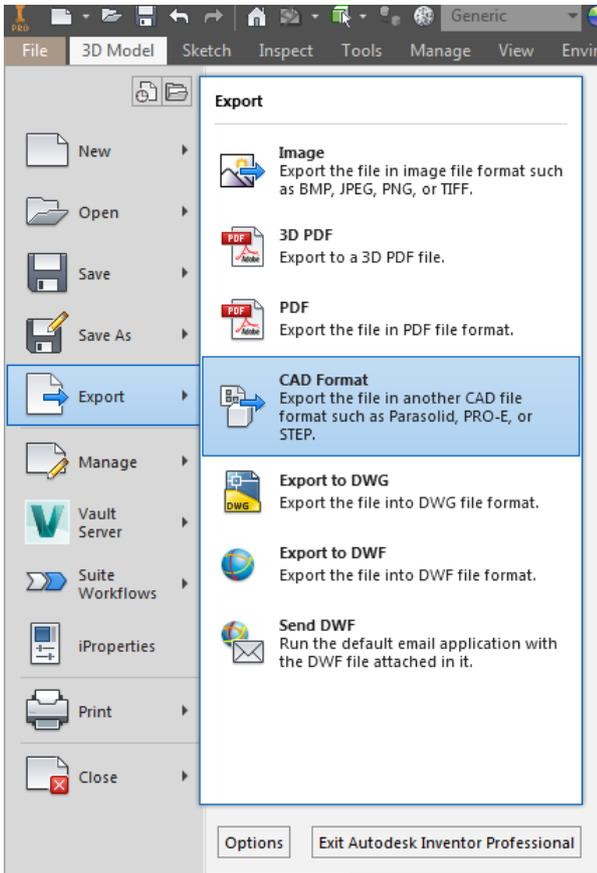
A new window will open, at bottom of page select 'Save as type', and then select 'STEP' using left key on mouse. Then select 'Save'.
