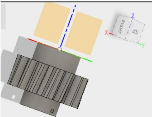
With Fusion 360 part needs to be assigned to home position on coordinates, this is start from 0 point of axis's. The Part still requires to be orientated in the XY plane. This can either be from beginning of modelling or on completion through the Move Function.
